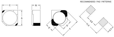
$\begin{array}{l} UNIT:mm/inch \\ A = 8.0 \pm 0.3 \ / \ 0.315 \pm 0.012 \\ B = 3.0 \ / \ 0.118 Max. \\ C = 8.0 \pm 0.3 \ / \ 0.315 \pm 0.012 \\ D = 6.5 \ / \ 0.256 \\ E = 3.0 \ / \ 0.118 \\ F = 10.5 \ / \ 0.413 \ Max. \end{array}$
